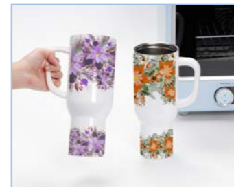
9 Take out the tumblers as the oven beeps after countdown finishes. Peel off the shrink film and sublimation paper; check the result;
