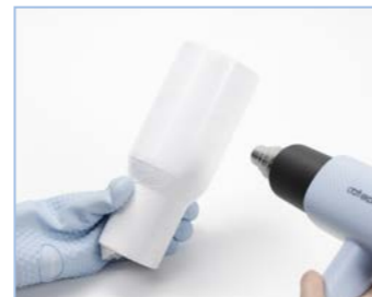
4 Use heat blower gun to shrink it and wrap the tumbler tightly;
